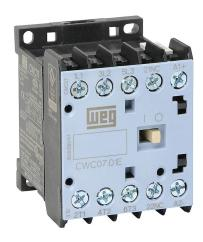
WEG Electric CWC series IEC miniature contactor, 7A, (3) N.O. power poles, (1) N.C. auxiliary contacts, 208-240 VAC (60Hz) coil voltage.
