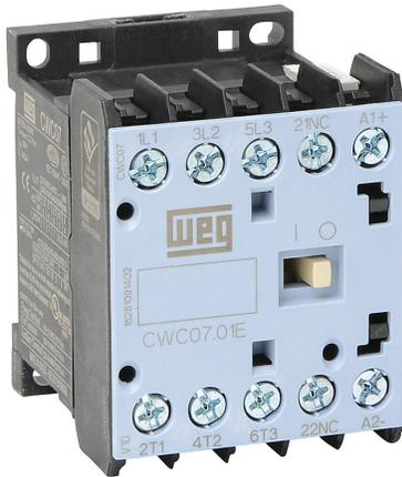
WEG Electric CWC series IEC miniature contactor, 7A, (3) N.O. power poles, (1) N.C. auxiliary contacts, 120 VAC (60Hz)/110 VAC (50Hz) coil voltage.
