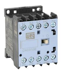
WEG Electric CWC series IEC miniature contactor, 7A, (3) N.O. power poles, (1) N.C. auxiliary contacts, 24 VAC (60Hz) coil voltage.
