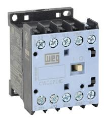
WEG Electric CWC series IEC miniature contactor, 7A, (3) N.O. power poles, (1) N.C. auxiliary contacts, 24 VDC coil voltage, low consumption.
