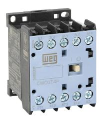
WEG Electric CWC series IEC miniature contactor, 7A, (4) N.O. power poles, 120 VAC (60Hz)/110 VAC (50Hz) coil voltage.
