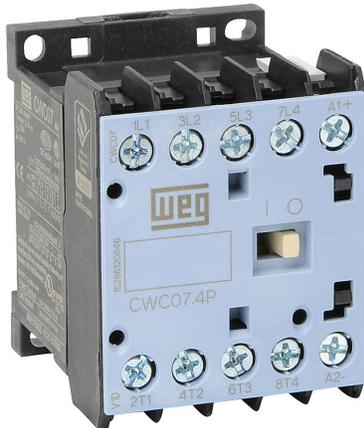
WEG Electric CWC series IEC miniature contactor, 7A, (4) N.O. power poles, 120 VAC (60Hz)/110 VAC (50Hz) coil voltage.
