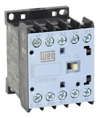
WEG Electric CWC series IEC miniature contactor, 7A, (4) N.O. power poles, 24 VAC (60Hz) coil voltage.
