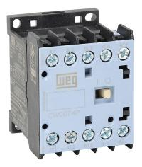
WEG Electric CWC series IEC miniature contactor, 7A, (4) N.O. power poles, 24 VDC coil voltage, low consumption.
