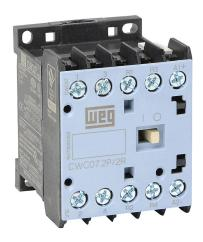
WEG Electric CWC series IEC miniature contactor, 7A, (2) N.O./(2) N.C. power poles, 120 VAC (60Hz)/110 VAC (50Hz) coil voltage.
