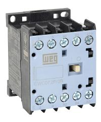
WEG Electric CWC series IEC miniature contactor, 7A, (2) N.O./(2) N.C. power poles, 24 VDC coil voltage.
