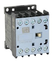
WEG Electric CWC series IEC miniature contactor, 16A, (3) N.O. power poles, (1) N.O. auxiliary contacts, 24 VAC (60Hz) coil voltage.
