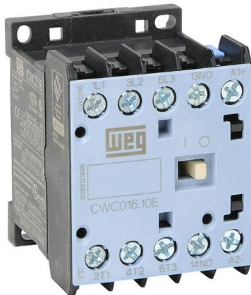
WEG Electric CWC series IEC miniature contactor, 16A, (3) N.O. power poles, (1) N.O. auxiliary contacts, 12 VDC coil voltage, low consumption.
