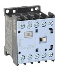
WEG Electric CWC series IEC miniature contactor, 16A, (3) N.O. power poles, (1) N.C. auxiliary contacts, 24 VAC (60Hz) coil voltage.
