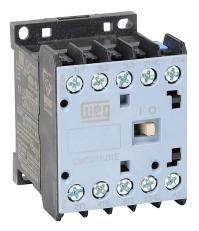
WEG Electric CWC series IEC miniature contactor, 16A, (3) N.O. power poles, (1) N.C. auxiliary contacts, 24 VDC coil voltage, low consumption.
