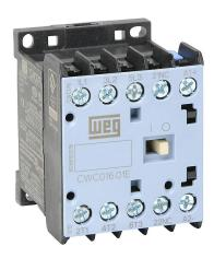
WEG Electric CWC series IEC miniature contactor, 16A, (3) N.O. power poles, (1) N.C. auxiliary contacts, 12 VDC coil voltage, low consumption.
