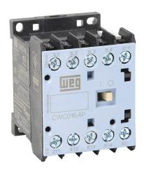
WEG Electric CWC series IEC miniature contactor, 16A, (4) N.O. power poles, 480 VAC (60Hz) coil voltage.
