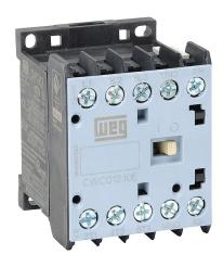
WEG Electric CWC series IEC miniature contactor, 12A, (3) N.O. power poles, (1) N.O. auxiliary contacts, 120 VAC (60Hz)/110 VAC (50Hz) coil voltage.
