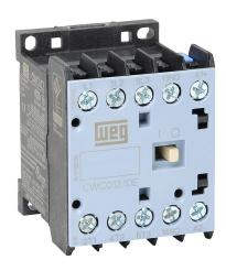
WEG Electric CWC series IEC miniature contactor, 12A, (3) N.O. power poles, (1) N.O. auxiliary contacts, 24 VDC coil voltage, low consumption.
