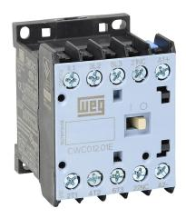
WEG Electric CWC series IEC miniature contactor, 12A, (3) N.O. power poles, (1) N.C. auxiliary contacts, 24 VDC coil voltage, low consumption.
