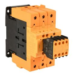
WEG Electric CWBS series IEC safety contactor, 95A, (3) N.O. power poles, (3) N.O./(3) N.C. safety auxiliary contacts, 110–255 VAC/VDC coil voltage, electronic.
