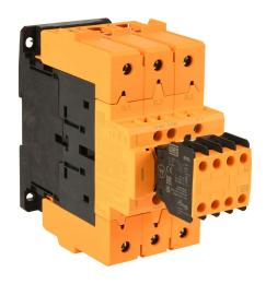
WEG Electric CWBS series IEC safety contactor, 95A, (3) N.O. power poles, (3) N.O./(3) N.C. safety auxiliary contacts, 24–60 VAC/VDC coil voltage, electronic.
