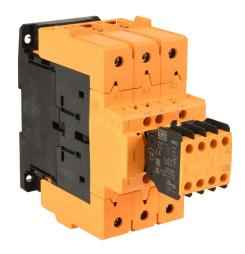
WEG Electric CWBS series IEC safety contactor, 95A, (3) N.O. power poles, (3) N.O./(3) N.C. safety auxiliary contacts, 120 VAC (50/60Hz) coil voltage.
