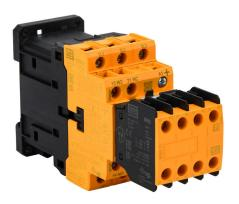
WEG Electric CWBS series IEC safety contactor, 9A, (3) N.O. power poles, (3) N.O./(3) N.C. safety auxiliary contacts, 24 VDC coil voltage.
