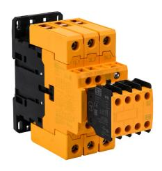
WEG Electric CWBS series IEC safety contactor, 80A, (3) N.O. power poles, (3) N.O./(3) N.C. safety auxiliary contacts, 120 VAC (50/60Hz) coil voltage.
