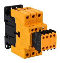
WEG Electric CWBS series IEC safety contactor, 80A, (3) N.O. power poles, (3) N.O./(3) N.C. safety auxiliary contacts, 24 VAC (50/60Hz) coil voltage.
