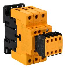
WEG Electric CWBS series IEC safety contactor, 65A, (3) N.O. power poles, (3) N.O./(3) N.C. safety auxiliary contacts, 120 VAC (50/60Hz) coil voltage.
