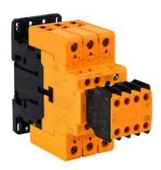
WEG Electric CWBS series IEC safety contactor, 65A, (3) N.O. power poles, (3) N.O./(3) N.C. safety auxiliary contacts, 24 VDC coil voltage.
