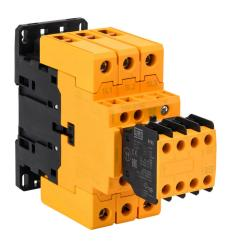
WEG Electric CWBS series IEC safety contactor, 40A, (3) N.O. power poles, (3) N.O./(3) N.C. safety auxiliary contacts, 120 VAC (50/60Hz) coil voltage.
