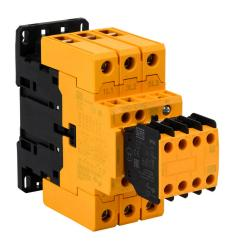
WEG Electric CWBS series IEC safety contactor, 40A, (3) N.O. power poles, (3) N.O./(3) N.C. safety auxiliary contacts, 24 VAC (50/60Hz) coil voltage.
