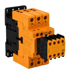
WEG Electric CWBS series IEC safety contactor, 40A, (3) N.O. power poles, (3) N.O./(3) N.C. safety auxiliary contacts, 24 VDC coil voltage.
