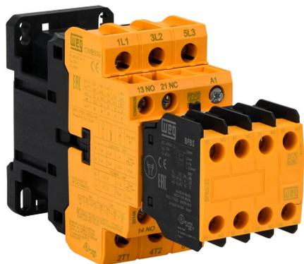
WEG Electric CWBS series IEC safety contactor, 38A, (3) N.O. power poles, (3) N.O./ (3) N.C. safety auxiliary contacts, 120 VAC (50/60Hz) coil voltage.
