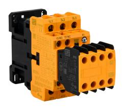
WEG Electric CWBS series IEC safety contactor, 38A, (3) N.O. power poles, (3) N.O./(3) N.C. safety auxiliary contacts, 24 VAC (50/60Hz) coil voltage.
