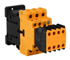
WEG Electric CWBS series IEC safety contactor, 38A, (3) N.O. power poles, (3) N.O./(3) N.C. safety auxiliary contacts, 24 VDC coil voltage.
