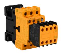
WEG Electric CWBS series IEC safety contactor, 32A, (3) N.O. power poles, (3) N.O./(3) N.C. safety auxiliary contacts, 24 VAC (50/60Hz) coil voltage.
