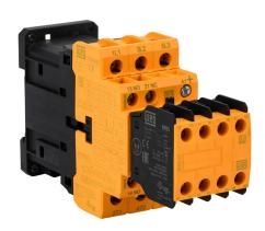
WEG Electric CWBS series IEC safety contactor, 32A, (3) N.O. power poles, (3) N.O./(3) N.C. safety auxiliary contacts, 24 VDC coil voltage.
