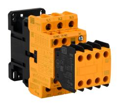
WEG Electric CWBS series IEC safety contactor, 25A, (3) N.O. power poles, (3) N.O./(3) N.C. safety auxiliary contacts, 24 VAC (50/60Hz) coil voltage.
