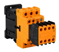
WEG Electric CWBS series IEC safety contactor, 25A, (3) N.O. power poles, (3) N.O./(3) N.C. safety auxiliary contacts, 24 VDC coil voltage.
