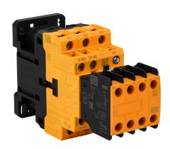
WEG Electric CWBS series IEC safety contactor, 18A, (3) N.O. power poles, (3) N.O./(3) N.C. safety auxiliary contacts, 24 VAC (50/60Hz) coil voltage.
