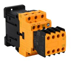
WEG Electric CWBS series IEC safety contactor, 18A, (3) N.O. power poles, (3) N.O./(3) N.C. safety auxiliary contacts, 24 VDC coil voltage.
