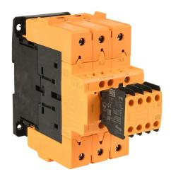
WEG Electric CWBS series IEC safety contactor, 125A, (3) N.O. power poles, (3) N.O./(3) N.C. safety auxiliary contacts, 110–255 VAC/VDC coil voltage, electronic.
