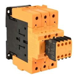
WEG Electric CWBS series IEC safety contactor, 125A, (3) N.O. power poles, (3) N.O./(3) N.C. safety auxiliary contacts, 24–60 VAC/VDC coil voltage, electronic.
