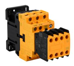
WEG Electric CWBS series IEC safety contactor, 12A, (3) N.O. power poles, (3) N.O./(3) N.C. safety auxiliary contacts, 120 VAC (50/60Hz) coil voltage.
