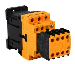
WEG Electric CWBS series IEC safety contactor, 12A, (3) N.O. power poles, (3) N.O./(3) N.C. safety auxiliary contacts, 24 VDC coil voltage.
