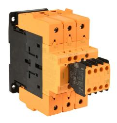
WEG Electric CWBS series IEC safety contactor, 110A, (3) N.O. power poles, (3) N.O./(3) N.C. safety auxiliary contacts, 110–255 VAC/VDC coil voltage, electronic.
