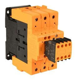
WEG Electric CWBS series IEC safety contactor, 110A, (3) N.O. power poles, (3) N.O./(3) N.C. safety auxiliary contacts, 24–60 VAC/VDC coil voltage, electronic.
