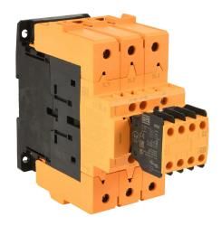
WEG Electric CWBS series IEC safety contactor, 110A, (3) N.O. power poles, (3) N.O./(3) N.C. safety auxiliary contacts, 120 VAC (50/60Hz) coil voltage.
