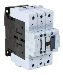
WEG Electric CWBN series IEC contactor, NEMA size 3, 95A, (3) N.O. power poles, (1) N.O./(1) N.C. auxiliary contacts, 120 VAC (50/60Hz) coil voltage.
