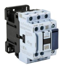
WEG Electric CWBN series IEC contactor, NEMA size 00, 9A, (3) N.O. power poles, (1) N.O./(1) N.C. auxiliary contacts, 480 VAC (50/60Hz) coil voltage.
