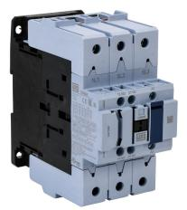
WEG Electric CWB series IEC contactor, 95A, (3) N.O. power poles, (1) N.O./(1) N.C. auxiliary contacts, 208 VAC (50/60Hz) coil voltage.
