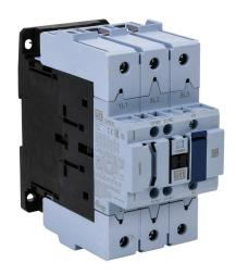
WEG Electric CWB series IEC contactor, 95A, (3) N.O. power poles, (1) N.O./(1) N.C. auxiliary contacts, 480 VAC (50/60Hz) coil voltage.
