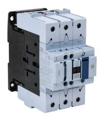
WEG Electric CWB series IEC contactor, 95A, (3) N.O. power poles, (1) N.O./(1) N.C. auxiliary contacts, 120 VAC (50/60Hz) coil voltage.
